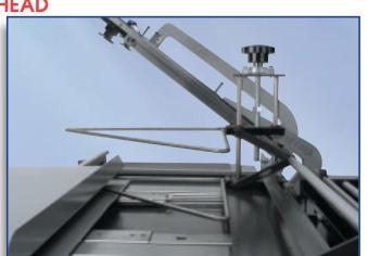
Unique design detaches the product tray from the inverting head, which simplifies film threading to a push of the film towards the seal area. The product trav is locked back in position and the pre-opened film is ready to accept product.
