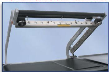
Hot Knife system features a continuously heated seal bar and is available on most Eastey Sealers. See HOT KNIFE DUOSEAL® BY REYNOLDS EASTEY brochure.
