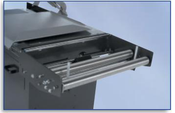
Simple positioning of the film roll provides quick, easy film adjustments and product changeover.
