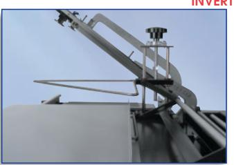
Inverting head allows the film to come off the back of machine. This pre-opens the film and minimizes operator effort which in turn increases output.
