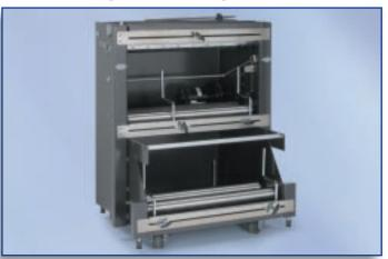
Power assisted rollers accommodate 2 rolls of film. Easy to follow film threading diagram shows how to guide film through the unwind. Effortless operation reduces operator fatigue and increases product output.
