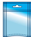
3 side seals stand-up bag with euro hole punch on vertical sealing bar and zip in line
