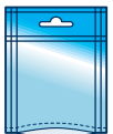
3 side seals bag stand-up (with euro hole punch on vertical sealing bar)
