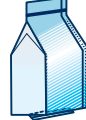
block bottom bag with off set vertical seal and cross web zip
